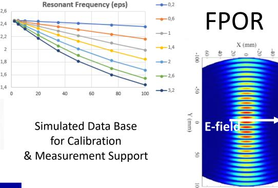
Field distributions obtained from full-wave EM simulations (QuickWave™ software by QWED).
